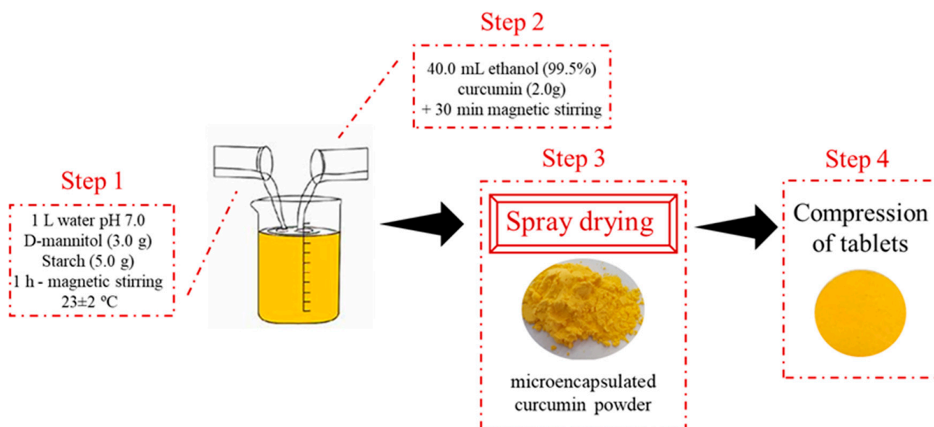
Figure 1. Method for producing microencapsulated curcumin formulations. Step 1: homogenization of starch and D-mannitol in water; Step 2: addition of curcumin in 99.5% ethanol; Step 3: drying the solution by spray-drying technique; Step 4: compression of the microcapsules into tablets.
